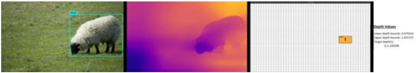
Fig. 5: Shown here is a good example of how the program can function given a semi-accurate depth map. The depth map produced a relatively good reading for the target which was about half of the range of the frame. This paired with the size normalisation produced a good representation of where the target should be placed.
