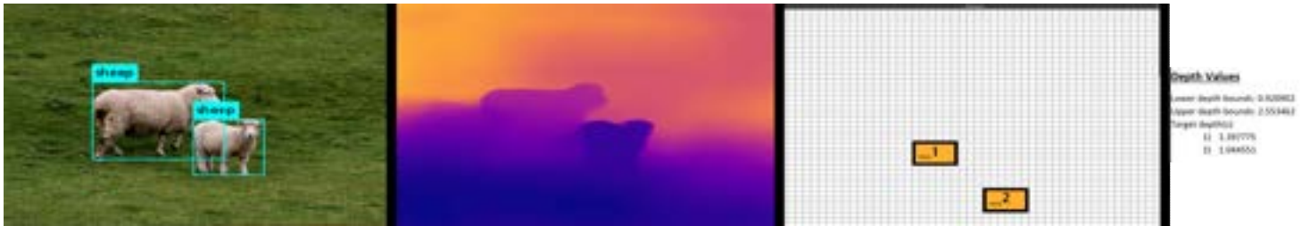
Fig. 6: It can be observed in this depth map that the targets have skewed the gradient of the image depth. This caused the target depth estimation to come up short causing the target position to be more forward than it should.
